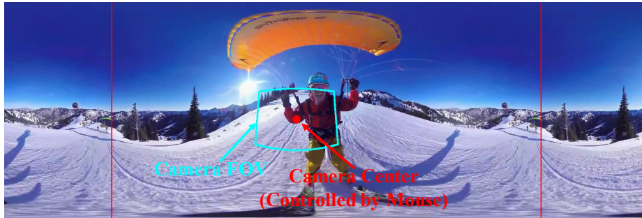
Fig. 4: The annotator controls the camera center using the mouse. The camera FOV is backprojected onto the 360° video during annotation to show the annotator what it captures.
